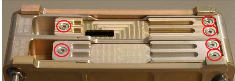
Figure 2.4 Countersunk screws for debug hatch covering the JTAG and Debug connectors.
